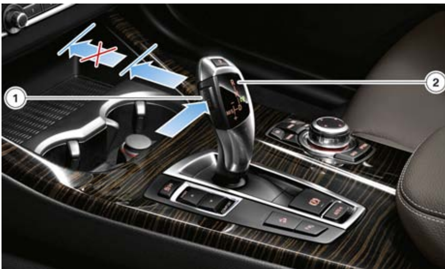
Electronic emergency release for GA8HP transmission, using F25 as example
